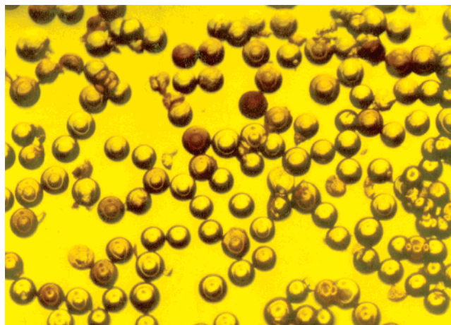
Figure 7. Example of screening assay between the triamine library and trisulfonated dye 2 using an optical microscope.
